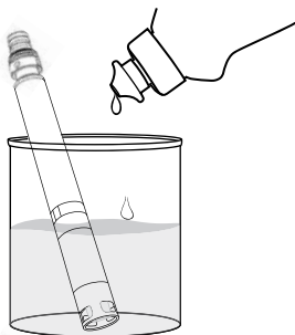
Figure 72 Cleaning the pH and pH/ORP sensor with dish soap
